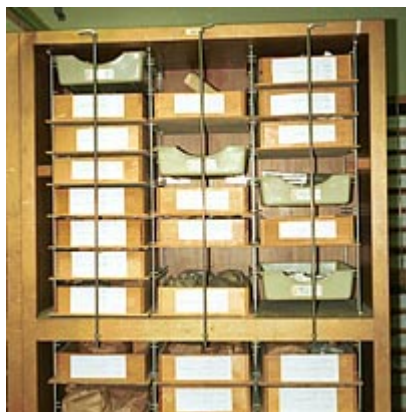
Drawer storage system for archeological artifacts. Note system includes security bar to ensure drawers stay in place during seismic activity. From the photograph collection of the U.S. Army Corps of Engineers, St. Louis District.
