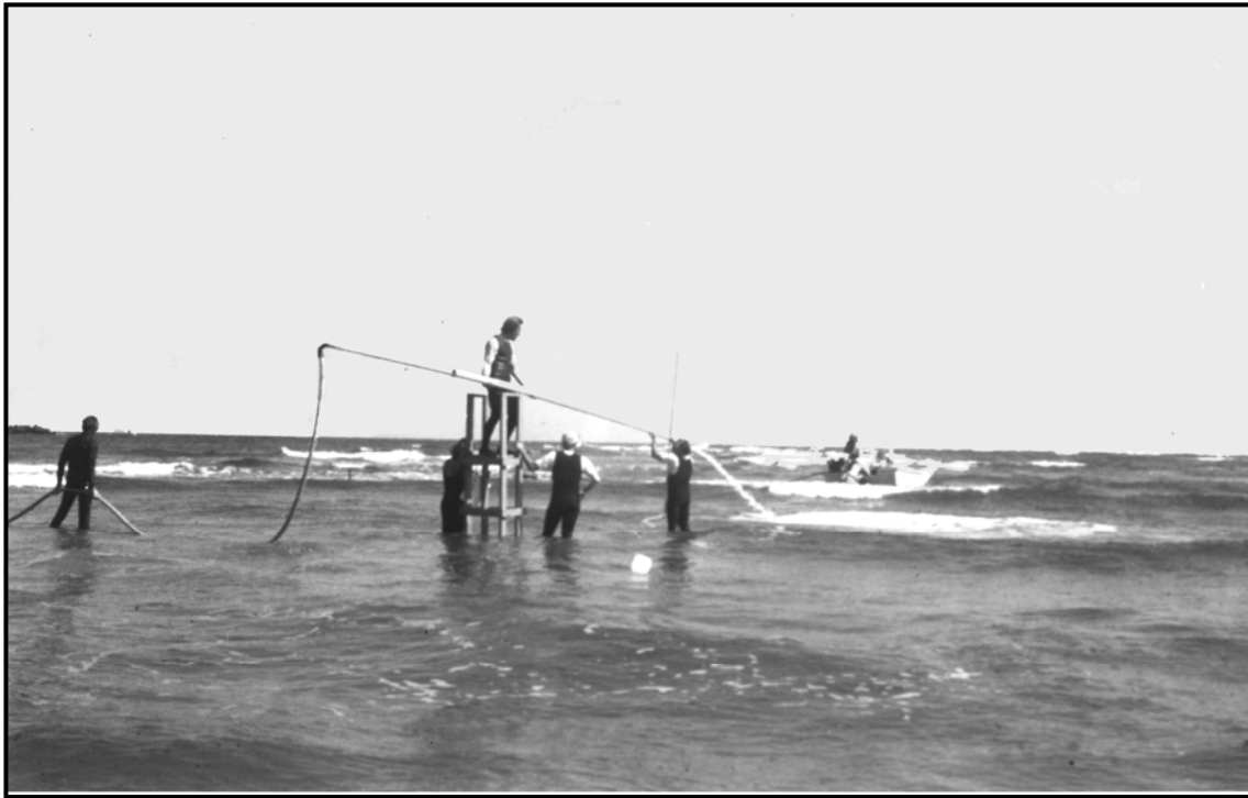
Figure 18: Investigation of magnetic anomaly targets using a hydrolic probe. Work took place in Masonboro Inlet as required through environmental investigation, Site 0001MBI
