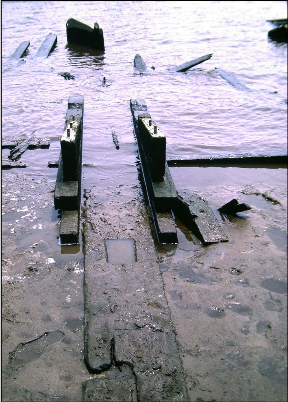
**Figure 16. Vessel remains (0029CFR), at low tide, looking east, showing keelson, engine bed timbers and iron rudder.**
