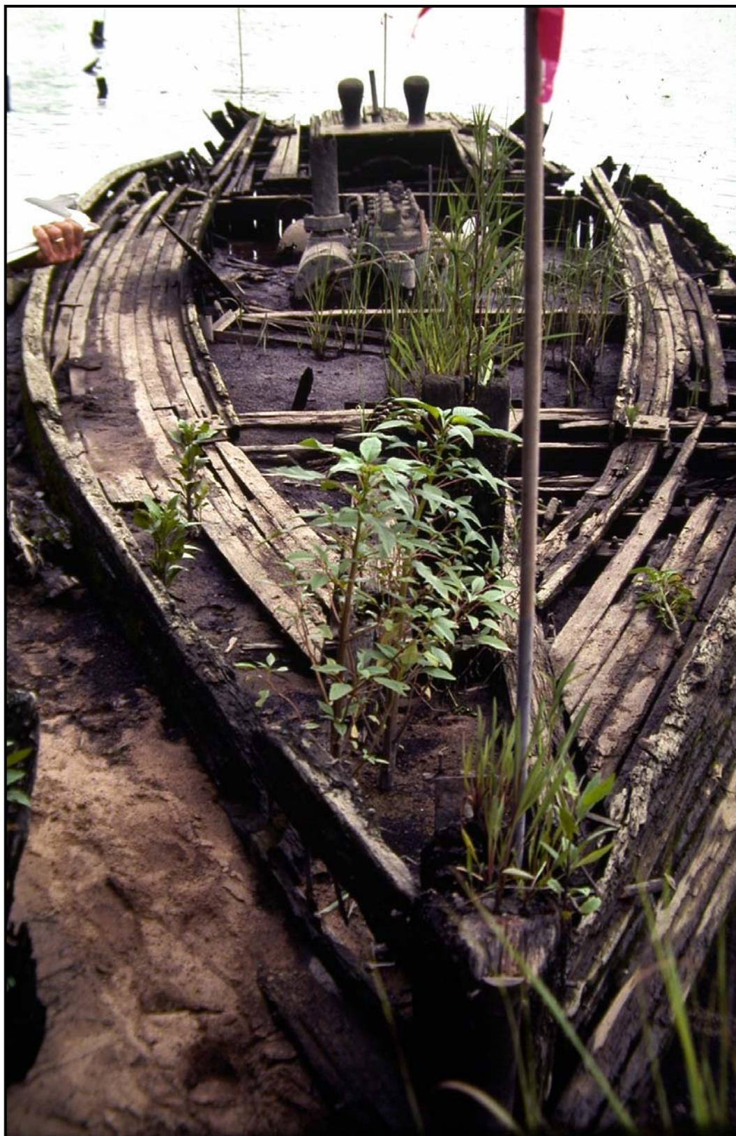
**Figure 12. Remains of *Stone 3* at low tide, looking east, with bow in foreground, showing 4-cylinder diesel engine and towing bitts.**
