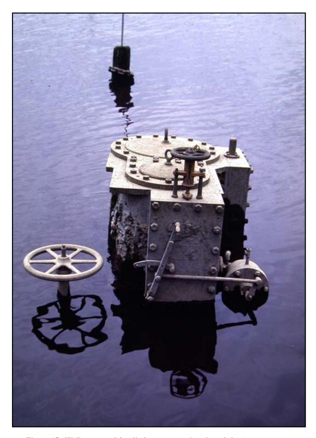
Figure 15. Well preserved 2-cylinder steam engine aboard the *Argonauta*.
