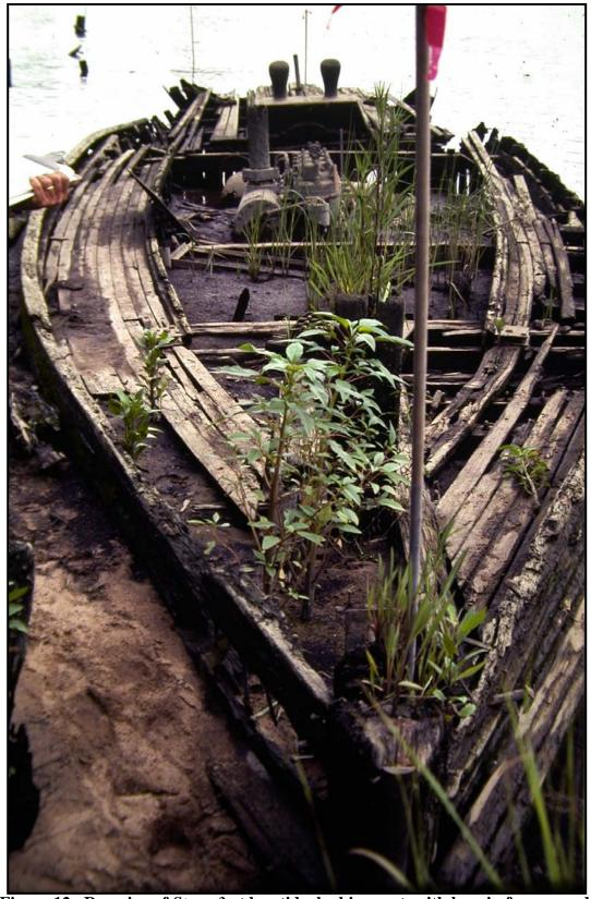
Figure 12. Remains of *Stone 3* at low tide, looking east, with bow in foreground, showing 4-cylinder diesel engine and towing bitts.
